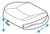
Pull control up to flip seatback to a forward flat position.
